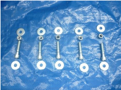
901486 SCHROEVEN M8x45 TCEI 901485 RINGEN 8,4x24 h2 901474 BORGMOEREN M8
